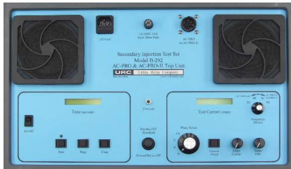
Figure 15.1: B-292 Secondary Injection Test Set
